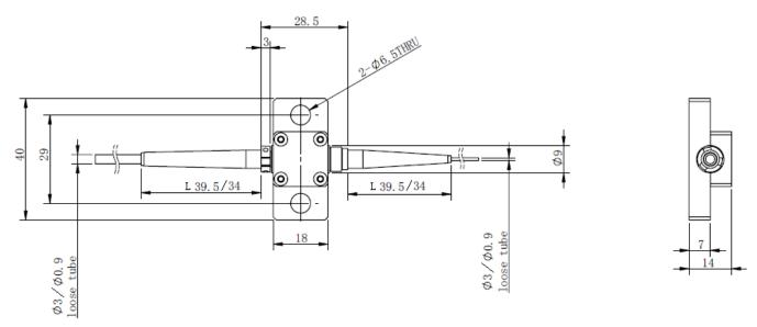
\*\*For  $\, \Phi \, 3mm$  loose tube , L=39.5mm; For  $\, \Phi \, 0.9mm$  loose tube , L=34mm;
